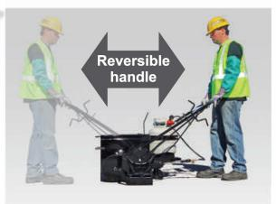
The new reversible handle feature allows the operator to change application direction "on the fly", increasing applicator versatility. By simply rotating the handle over the unit, the application direction is reversed. Regardless of where repair is located, operator can maneuver applicator from safest possible position. This feature brings more functionality and ease of operation, while adding operator safety.
